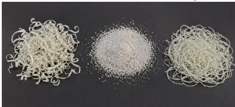
Figure 4. Types of chips formed during the machining of glass fiber reinforced composites: (a) fragmented chips, (b) powder-like chips, and (c) continuous chips.
