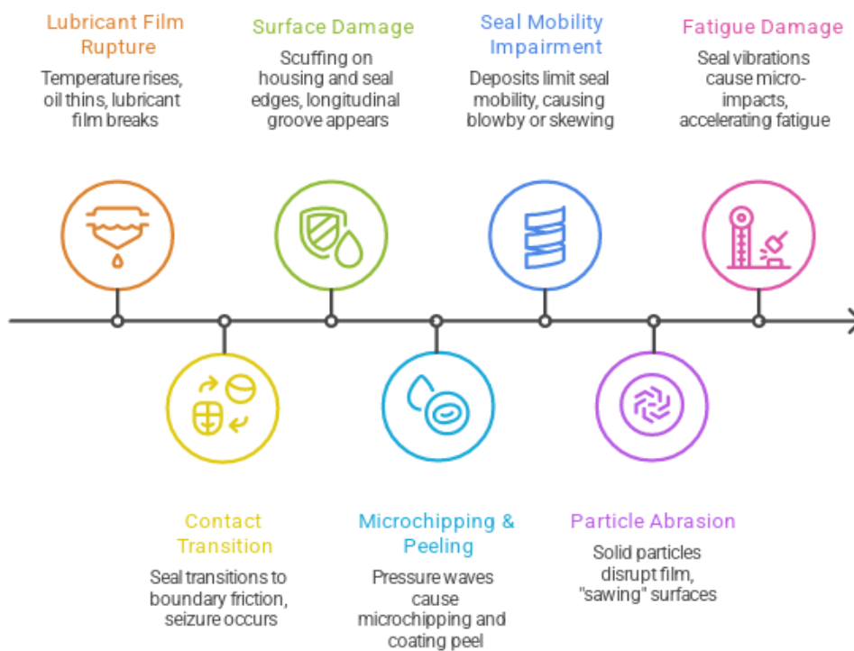
Fig. 2. Seal Failure Pathways Under High Load
