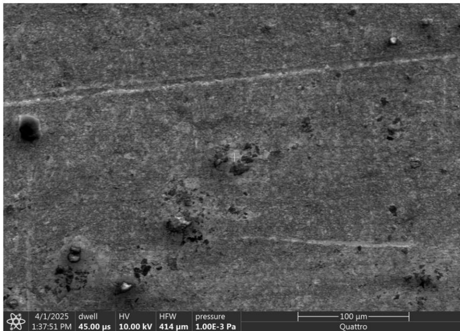
Fig. 1b SEM image of a steel surface protected by the Renox antiwear additive (pitting sites)
