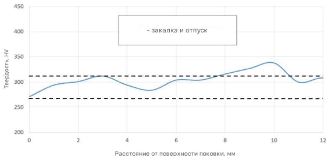
Fig. 8. Changes in hardness (HB) across the cross-section in the selected measurement plane for a product that was oil quenched and tempered.
