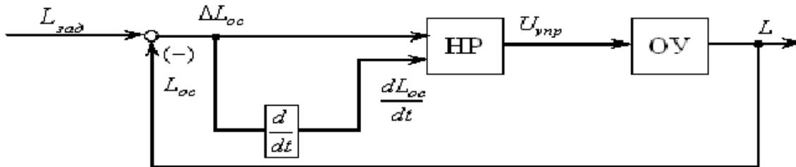
Fig. 1. Simplified block diagram of the SEP ACS with a fuzzy 1 controller
