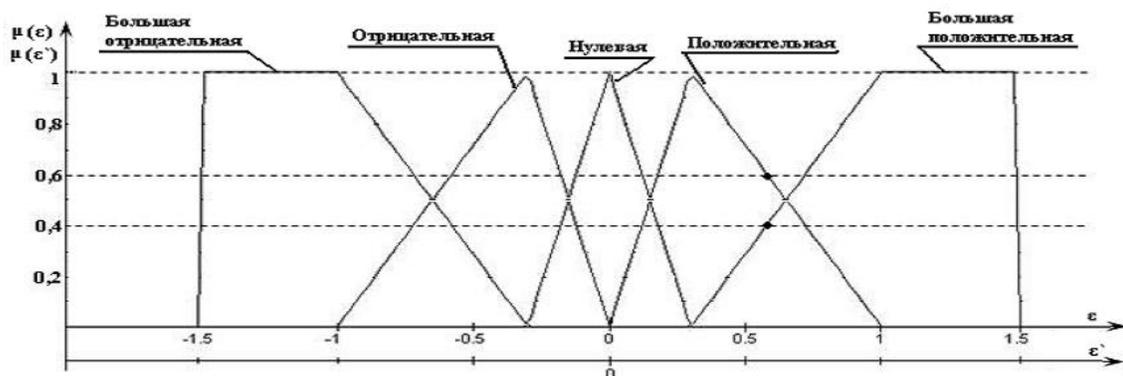
Fig. 2. Fuzzification of the error and the rate of change of the error.
