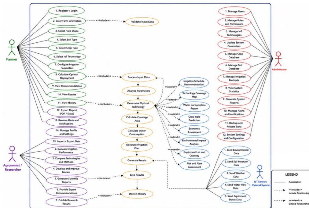
Figure 5. Use case diagram of an IoT-based sensor placement and irrigation planning system for agriculture
